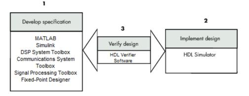
As the figure shows, HDL Verifier software connects tools that traditionally have been used discretely to perform specific steps in the design process. By connecting these tools, the link simplifies verification by allowing you to cosimulate the implementation and original specification directly. This cosimulation results in significant time savings and the elimination of errors inherent to manual comparison and inspection.
